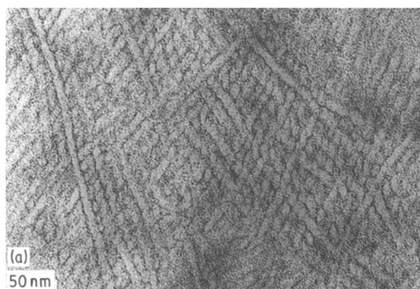
Figure 7 Electron micrographs of spherulite sections in the weld line at (a) T_w = 100^\circ\text{C} and (b) T_w = 120^\circ\text{C} .
